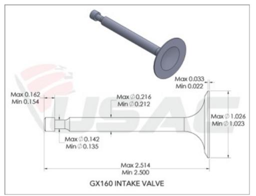
2. Drawing of valve dimensions (Intake Valve followed by Exhaust Valve)
