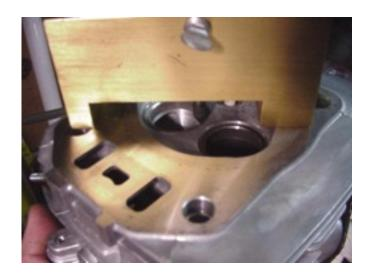
3. Measure from surface of head to lowest machined area in the bowl of the port. This dimension will be:
