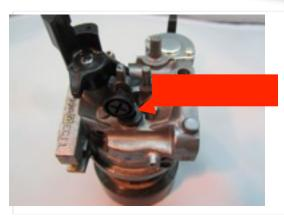
Remove the idle adjustment screw and then carefully pry up on the **Pilot Air Jet** to remove.
